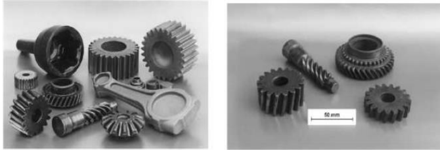
Figure 4. Spur, helical, bevel and worm gears, connecting rod and overhead camshafts joints - NNS forged (Doege and Bohnsak (2000))
