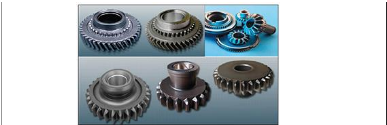
Figure 1. Near net formed gears: final form with finished teeth. (Dean, 2000)
