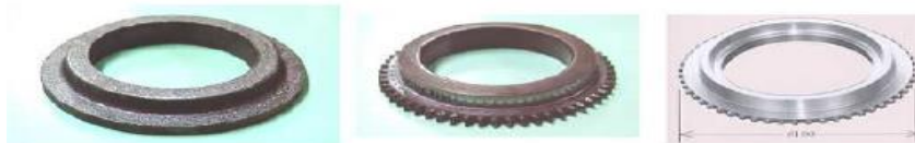
Figure 8. Synchronizer cone ring: cold forging steps.
